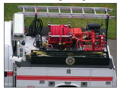
Brush 17 significantly increases the wild-land and brushfire fighting capabilities of the City of Renton and Fire District 40 during the high-risk seasons. When the equipment is not needed, it can be removed from the truck and moved in and out of any fire station with its own lift system, making it portable and storable. The truck then serves other purposes such as assisting the city's dive team and towing the city's 4 wheel drive all terrain vehicle.
